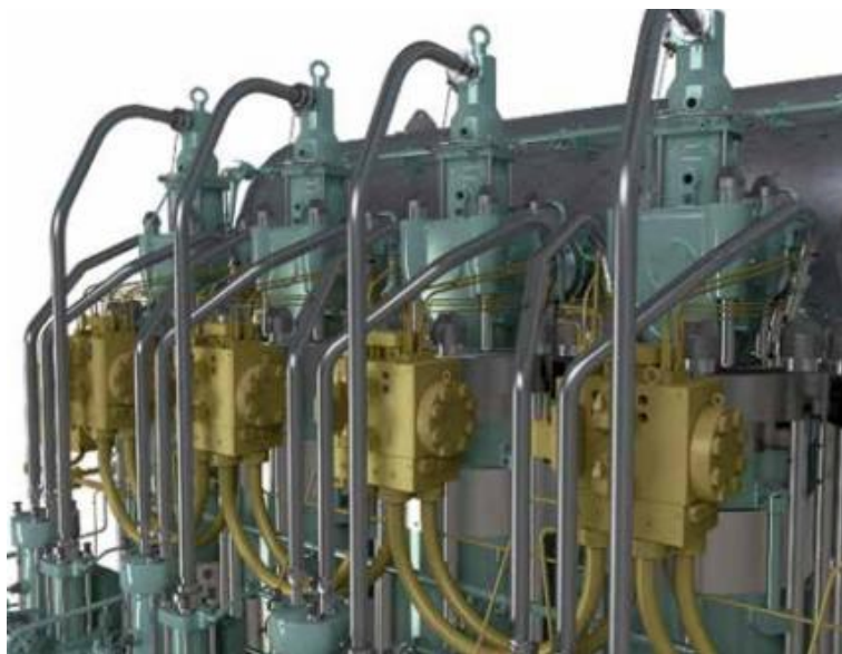
Fig. 6. New engine gas supply module.
